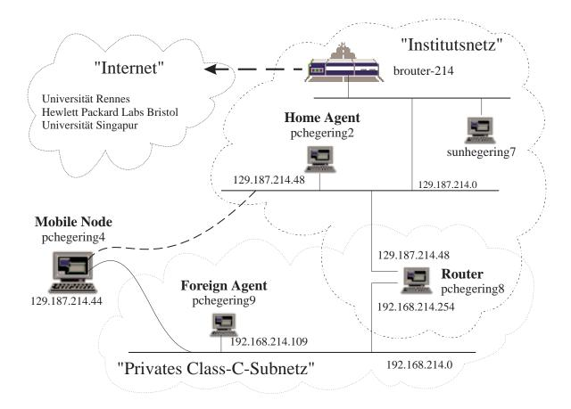
Figure 2: The Mobile-IP Testbed at the University of Munich (in German)
