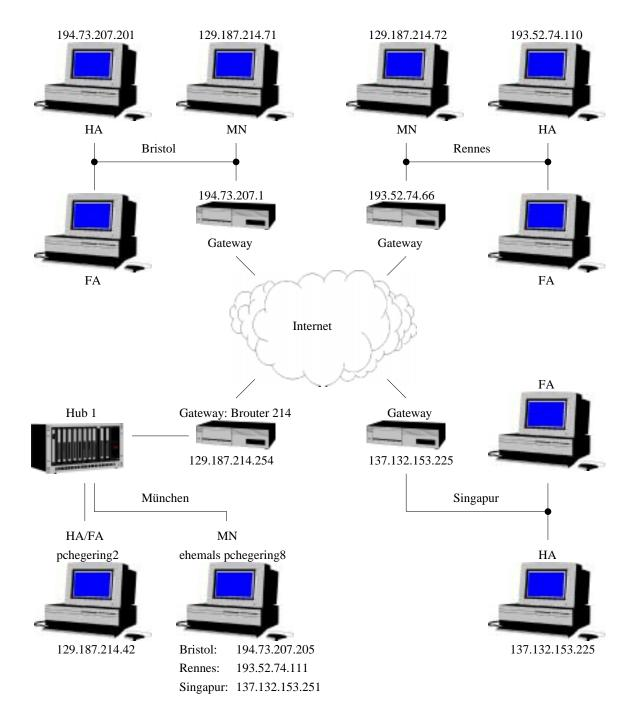
Figure 1: The Mobile-IP Testbed of the HP Labs and the Universities of Rennes and Munich (in German)
