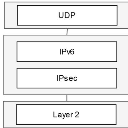
Figure 4.2.: Protocol stack with integrated IPsec implementation.
