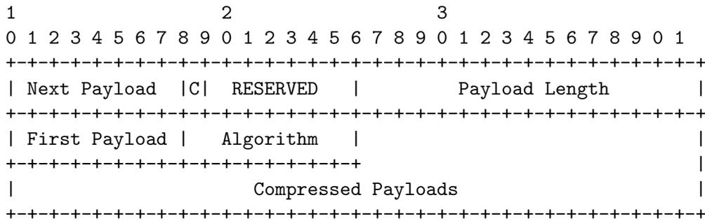
Figure 4.6.: IKE Compressed payload header as proposed in [Smy20]
