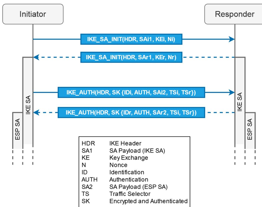
Figure 5.1.: Sequence diagram for the IKE Initial Exchanges.
