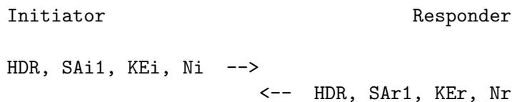
Figure 2.4.: IKE\_SA\_INIT exchange without optional payloads [KHN<sup>+</sup>14]
