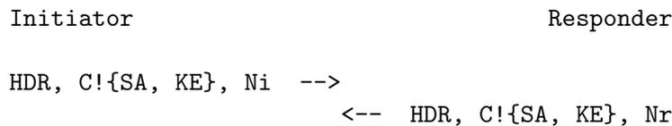
Figure 4.7.: Compressed IKE\_SA\_INIT exchange without optional payloads as proposed in [Smy20]
