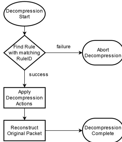
Figure 5.5.: SCHC Decompression Sequence
