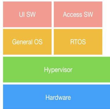
Figure 3.3: RTOS coexisting with general-purpose OS.
