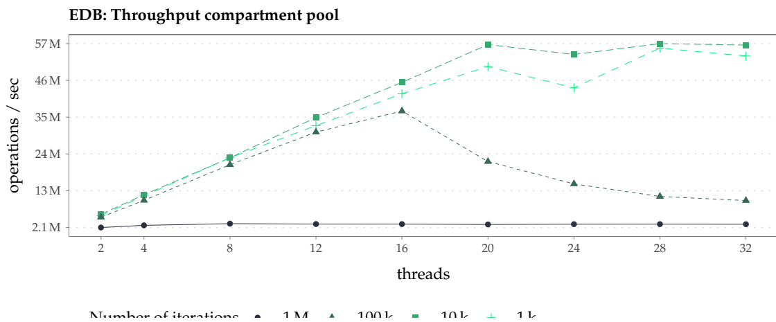
Figure 2.11: Throughput of wait-free array-based compartment pool in scenario enqueue/dequeue-bulk with K = 5 , by number of iterations
